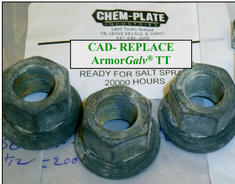
Wheel Nuts after 2,000 hours of salt spray. Flange turns freely even with corrosion product present - just like Cad!
